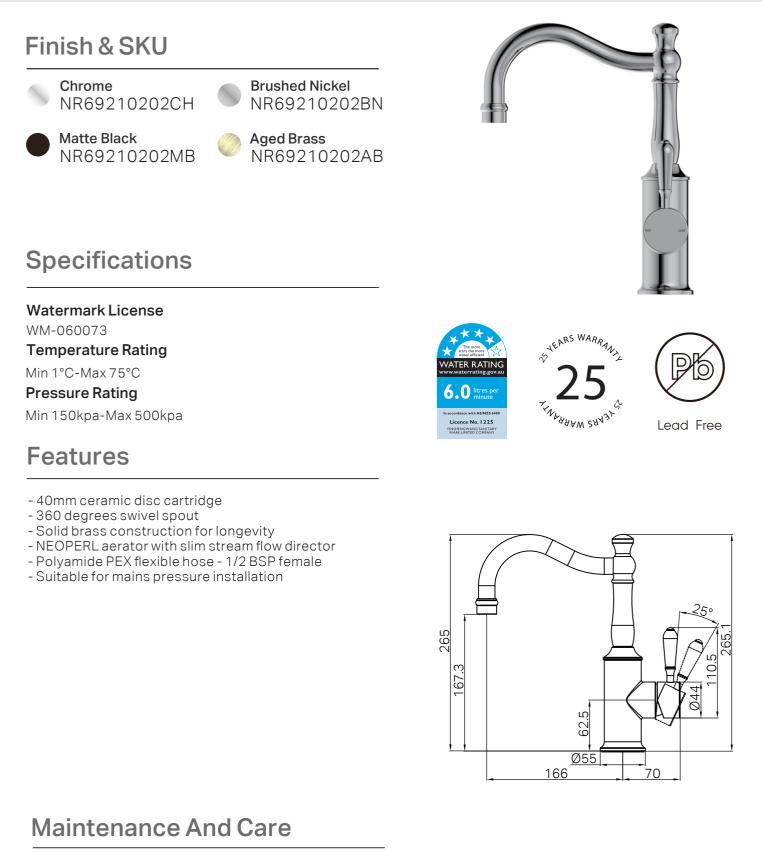
Regularly check the mixer and connections for signs of wear or leaks.
