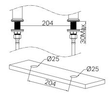
1. Pre-drill or create two holes with diameter of 25mm at the proper location. Please note that the thickness of the surface should be between 3mm-30mm and the distance of two holes is 204mm.
