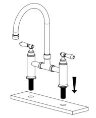
2. Inset the mixer body and pass it through the hole in the counter-top.
