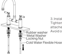
3. Install the rubbers, metal washers and locking nuts.
