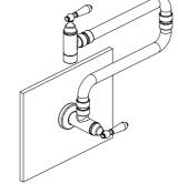
5. Turn on the water supply, and inspect all connections for any signs of leakage
