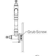
4. Screw the pot filler body by tightening the two grub screws using an Allen key, and push the plate onto the wall. (Ensure the screws are tightened firmly but do not over-tighten.)
