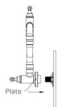
3. Push the plate back to the pot filler body, and screw the pot filler body onto the G1/2 outlet.
