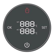
If the electronic instant hot water appliance is empty of water and is turned ON then this will be automatically sensed, the heating element will not energise and the "lack of water" indictor will be flashing on the display panel shown by the flashing of the E3
