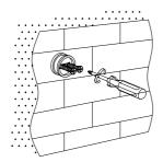
4. Place the fixing block covers over the holes and secure them firmly with expansion screws.
