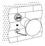
5. Install the robe hook onto the mounting bracket and secure it by tightening the grub screw.
