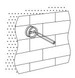
1. Use the mounting bracket to mark the drilling points on the wall.
