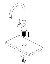
2. Place the mixer body and pass the Pex hoses through the hole in the counter-top. Ensuring the O-RING sits within the bottom groove of the base plate to prevent water leakage through the cabinet.
