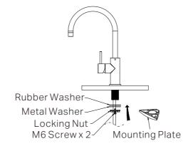
3. Install the rubber and metal washers, if a mounting plate is required, install the mounting plate after placing the rubber
