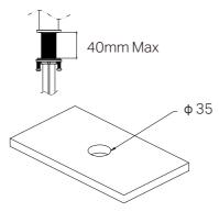
1. Pre-drill or create a hole with a diameter of 35mm at the proper location. Please note that the thickness of the surface should be between 3mm-40mm.
