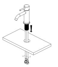
2. Place the mixer body and pass the Pex hoses through the hole in the counter-top. Ensuring the O-RING sits within the bottom groove of the base plate to prevent water leakage through the cabinet.
