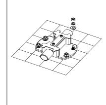
5. Connect hot and cold water according to the diagram, check whether there is leakage, and then lay cement and tile according to the diagram.
