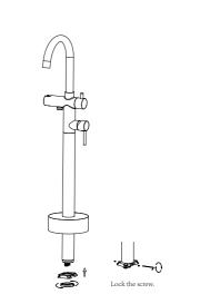
9. Push floor standing mixer into the base plate. Red water connector into H. Blue water connector into C
