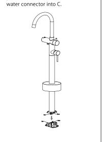
**10.** Fix mixer into base plate with supplied screws using Allen key.
