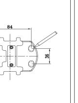
2. Drill holes according to the drawn mark, with a diameter of 10 mm and a depth of 45 mm.
