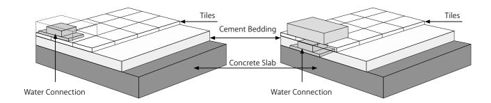
**1.** Draw the pre-drilling position in pencil on the floor.
