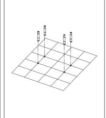
4. Discuss with your plumber/installer how the plumbing will be run, if elbows are needed we recommend installing to body now.
