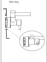
5. Tighten the grub screw with the
