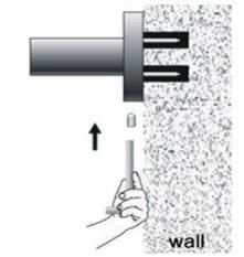
5. Screw grub screws into the base, make it against to the fixing block tight and firm.
