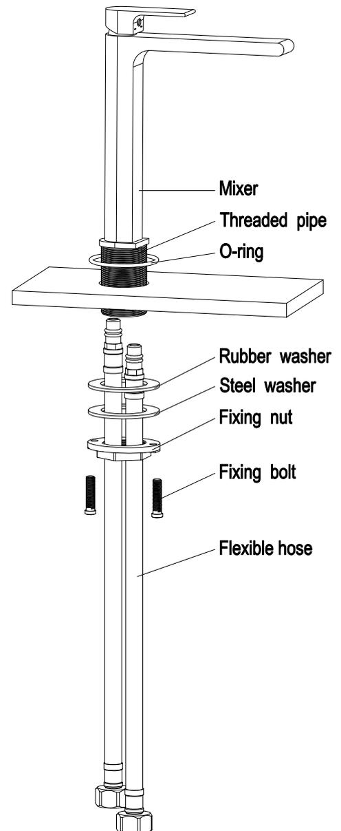
1. Screw the flexible hoses into the mixer body, and fully hand tighten.
