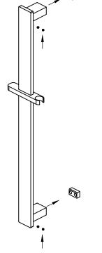
6. Install shower rail onto brackets, tighten four grub screws by hex wrench.
