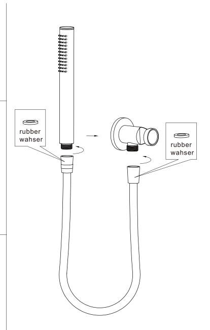
4. Connect bracket and hand shower with hose. TEST & CHECK FOR LEAKS.
