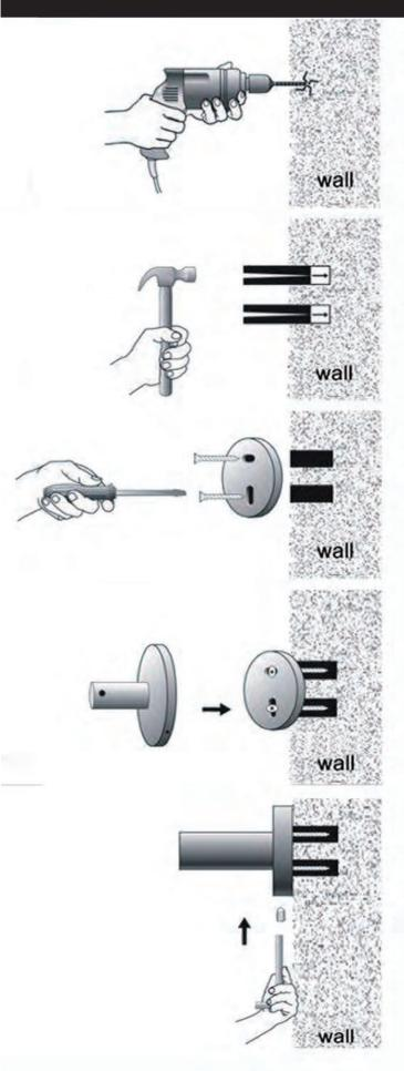
1. Put the fixing blocks (piece) over on the right place on the wall, and stay level, use marking pen through the holes of fixing block to mark out fixing spots on the wall. Then drill holes by electric hand drill with 6mm drilling bit on the spots.
