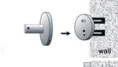
4. Put the base of bathroom accessory cover on the fixing blocks.
