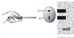
3.Put fixing block cover on the holes and fix firmly by expansion screws.
