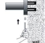
5. Screw grub screws into the base, make it against to the fixing block tight and firm.
