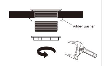
2. Put the thread pipe through the bath hole. Fit the rubber washer and tighten up the nut on thread pipe by screw driver.
