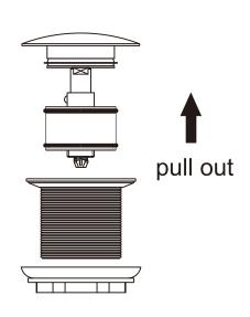
1. Disassemble pop -up waste by pulling out the cap.
