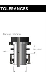
MIN: 34mm MAX: 42mm Hole Diameter
