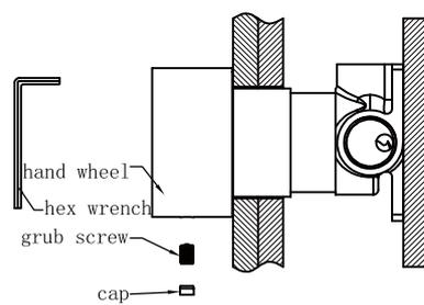
7. Make hand wheel cover on connecting rod, tighten grub screw of hand wheel by hex wrench, put cap into hand wheel.
