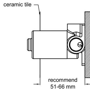
1. Fix body on noggin and ensure installation depth is 51-66mm from noggin to ceramic tile.
