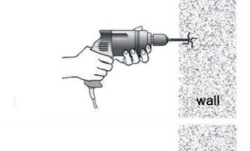
1. Put the fixing blocks (piece) over on the right place on the wall, and stay level, use marking pen through the holes of fixing block to mark out fixing spots on the wall. Then drill holes by electric hand drill with 6mm drilling bit on the spots.
